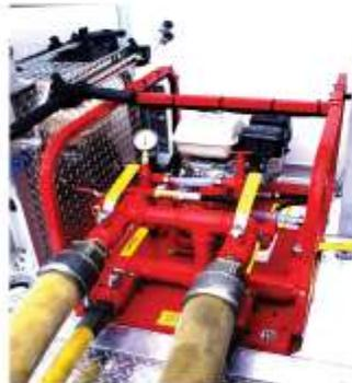
Designed to safely test fire hoses up to 6" in diameter, our **Draft Commander Fire Hose Tester** can be mounted on the Draft Commander and can be removed to operate independently.
