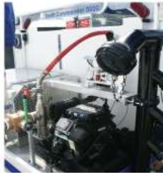
The **Draft Commander 300GPM Transfer Pump Unit** is designed to allow the Draft Commander to be used as a stationary water supply, transferring water to firefighting units.
