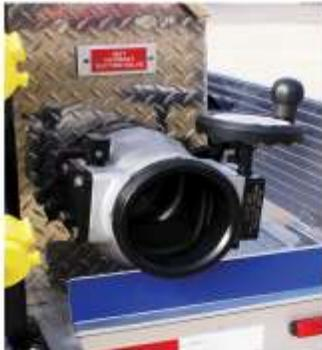
The **6" Wet Hydrant with Suction Valve** is used during fire pump engineer training to enable the flow of water without using a primer on the fire engine.
