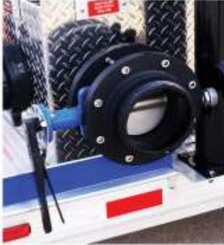
The **6" Vacuum Butterfly Suction Valve** is used when performing the tank to pump flow test, and is also used during firefighter engineer training.
