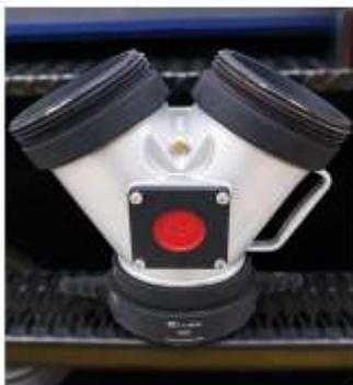
The specially designed **Siamese valve** is for pump testing 1750 GPM (max. of 2000 GPM) from one side of a fire apparatus. (6" NST swivel female LH by NST male by 6" NST male.)
