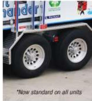
The **Custom Aluminum Wheels** can be included as an alternative to the standard rims, preventing corrosion and providing much greater longevity than its steel counterpart. They come in an attractive, clean-cut style.
